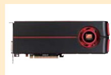
ATI Radeon HD 5870 GPU 雙精度浮點運算達2.72 TFLOPS，單精度浮點運算達544 GFLOPS
